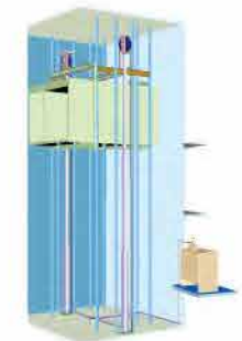
Double-cylinder side action 6-rail 2 : 1
